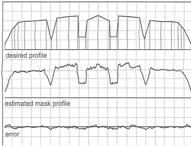
Figure 8. The desired profile and the profile produced by the net for k = 9 , \delta = 4 . For visualization purposes, the y -axis (the profiles and the error) scaling is enlarged 3 times compared to the x -axis. One can clearly see that the error is especially increased in the neighborhood of strong changes in the profile.
