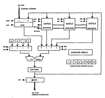
FIG. 9 BLOCK DIAGRAM FOR Z SCAN DECODER (DATA SECTION)..
