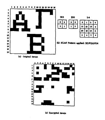
Figure 6: The SCAN transposition cipher applied on a binary image.
