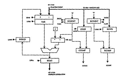
FIG. 5. BLOCK DIAGRAM OF RASTER SCAN DECODER (DATA SECTION).
