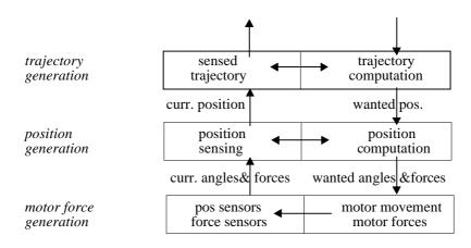
Fig. 9 The robot control layers
