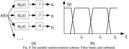
Fig. 8 The parallel multiresolution scheme: Filter banks and subbands for multirate sampling
