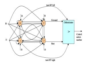
Figure 10: A neural network controller with 4 neurons (outputs), evolved by AEA.
